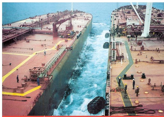
Fig. 4 Application of fenders to 300,000 DWT class Tanker
