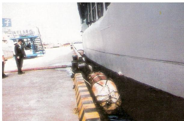
Fig. 7 Application of fenders to a quay of naval harbor in Shanghai
